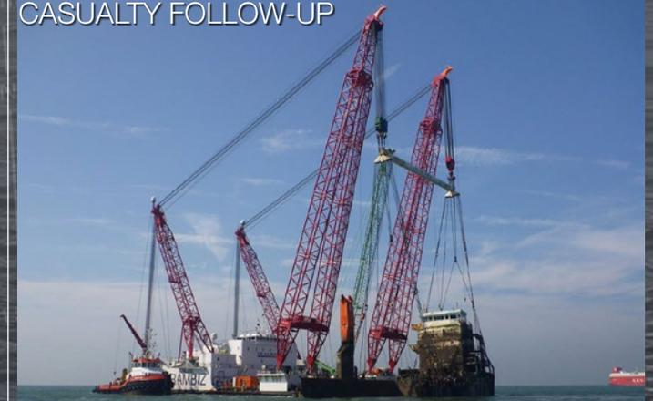
**Flinterstar** - editions 132, 133, 134, 135, 139, 140, 152, 161, 165, 169 & 170 - the removal of the wreck has been completed ahead of schedule with the aft section having been transported to Gent for recycling on the Scaldis-sheerleg Rambiz. Normal maritime traffic can now resume and the exclusion zone for pleasure and fishing boats has been lifted.
